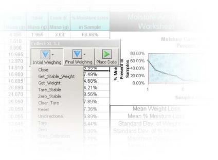
When you start Collect XL, it will ask you to select a predefined Method. Making the selection will automatically start Excel®, load the correct Excel® template and add an instrument control menu. Excel® is ready to be used in the normal manner to enter data, draw graphs, run macros, create reports, load files or control instruments.
